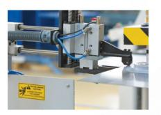
Sheet Thickneess Measurement System
