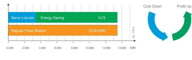
AD-Servo Press Brakes Regular Press Brakes
