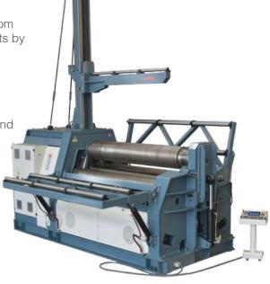
Especially the during bendings of the large diameter and thin metarial ellipse, paralel corners and polycentric shaped may effect the precisions and can cause deformation of the metarial, when there is not enough support
